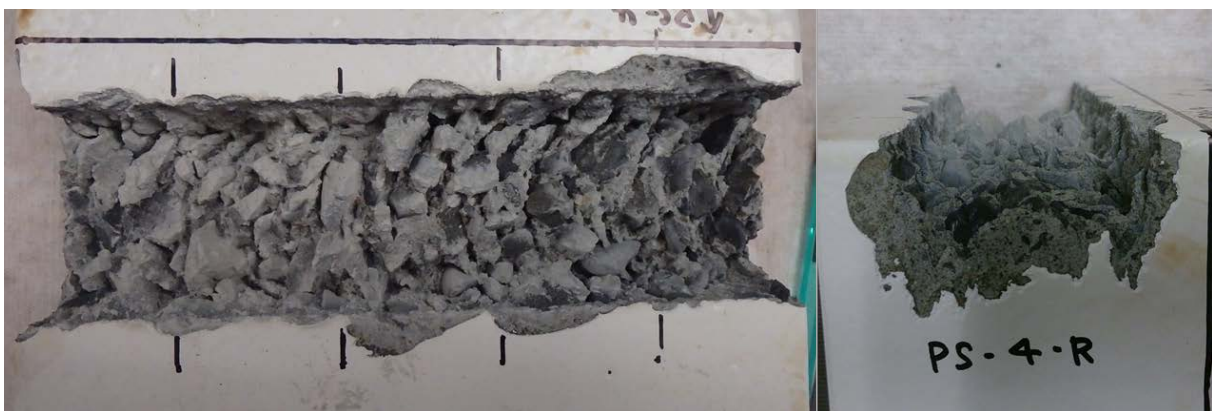
Fig. 4. Scabbled Pass of Painted Concrete
